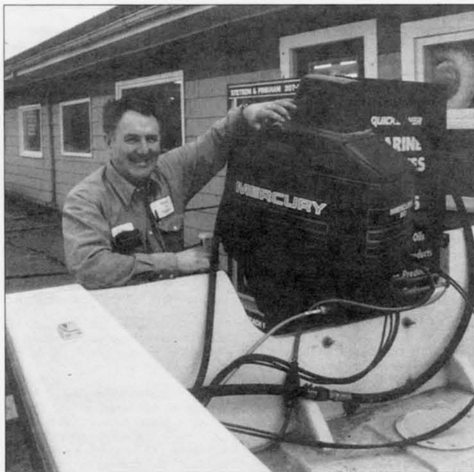
HOUSED ATOP THIS MERCURY is an outboard-powered hydraulic pump, which runs a hauling sheave. The pump can be put to use on outboards above 40 hp.
