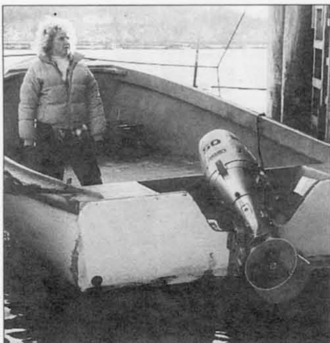
THE HANDLER nozzle fits over an outboard's prop. The prop-nozzle combination provides additional thrust.
